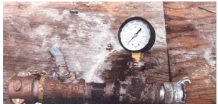
4. Coupling with on/off valve and pressure gauge.
